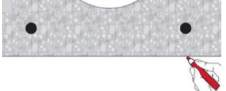
3. Marking pre-stressed steel position
