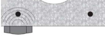
3. Marking pre-stressed steel position
